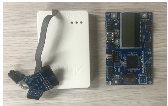
Fig. 5. In-circuit debugger; Atmel Ice & XMEGA-A3BU Xplained
